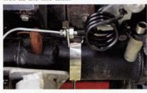
11. A braided hose runs from each caliper to the line tab where it connects to the hard line. The line tabs are held in place by stainless steel band clamps, saving the need to weld on the rearend housing.
