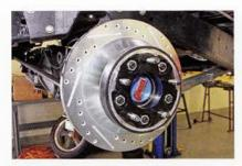
18. Next the four axle retaining bolts can be tightened and the rotor can be installed. I'm using Trans Dapt wheel spacers in the rear to get the track width in line with the front, which can be seen mounted to the
