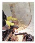
15. I did this using a Lincoln plasma cutter with a piece of scrap sheetmetal protecting the bearing.
