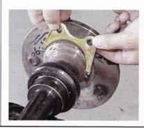
14. The flange plates that secure the axles in the housing are installed onto the axles before the bearings are pressed into service. If you don't want to press off the bearings to remove them, you'll have to cut the flange plates off.
