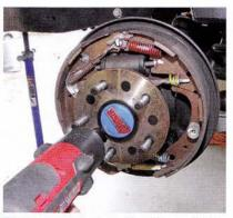
33. The four bolts that attach the backing plate to the axle housing are accessible through a hole in the axle flange. Remove these four bolts and the axle followed by the brake can be slid right off the housing.
