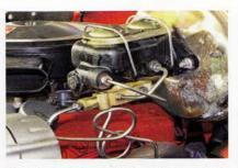
112. The last step of the install is to install the new disc/disc proportioning valve in place of the old. This ensures that both the front and rear brakes receive the proper pressure needed for a safe stop.
