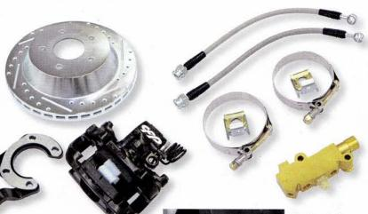
11. To do the drum to disc swap, we ordered up everything needed from CPP including drilled and slotted rotors, calipers, brackets and shims, steel braided hose, line clamps, steel brake lines, and a disc/disc proportioning valve.
