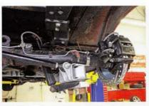
110. Since the hard lines on the rearend went from the junction block to the wheel cylinders, they either need to be shortened or replaced. I opted to use CPP's rear line kit that comes with the axle brackets as well as the line tabs.
