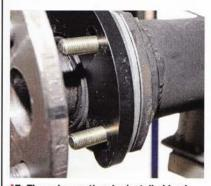
17. The axle can then be installed back in the housing before the caliper bracket is slid into place. Notice the relationship between the caliper bracket (black) and the special shim (silver). This is required to retain the proper bearing preload and to secure the axle.
