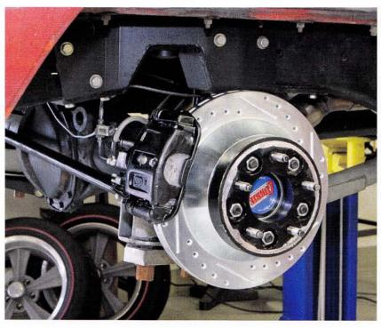
power, the C10 managed to improve upon its 60-0-mph brake test from 189 feet down to 148 feet, not bad for an afternoon's worth of work. With a nice set of sticky tires and with the shortbed conversion complete, we're hoping to get that number down even lower. Stay tuned!
