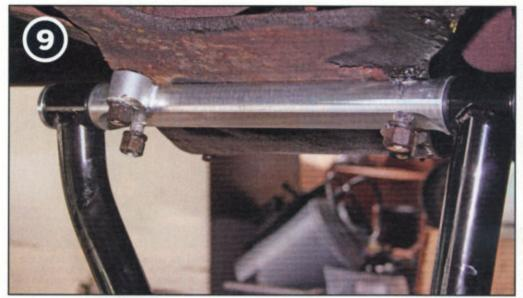
The lower control arm mounts flush to the underside of the frame and simply get tightened using four bolts and lock washers. Try to tighten these bolts at the same time ensuring that the control arm mounts flush. If you were to tighten one side and then the other, you run the chance of it getting kinked and ultimately coming lose down the road.
