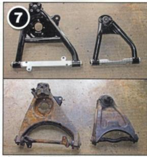
▲Check out our CPP upper and lower control arms next to the factory set. The strength of 1.25-inch tubular control arms will add rigidity to the suspension, give it five degrees of added caster, and improve ride quality tenfold. Also, the thick mounting/pivot arms on both the upper and lower mounts use the existing hardware. Try not to lose the shims that came out of the upper control arm from the last alignment. Shops will have these but it's good to know how the car was set up before hand.
