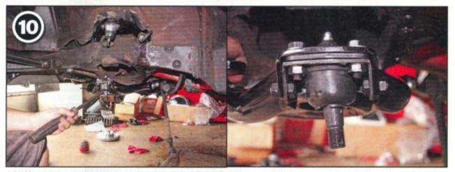
▲At this point, our control arms are in place. Already installed by CPP, the new ball joints come pre-greased and provide a noise and vibration-free ride. Also, the kit comes with all the castle nuts, cotter pins, and dust boots to finish the job. As a precaution, use a grease gun to make sure they do not need any more lubrication. Better to be safe than sorry here.
