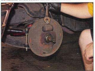
The factory drum brakes were completely shot, so our timing could not have been better. (See our upgrade story on page 52 to see how we added front discs.) Next, I removed the springs holding the pads in place, which simply allowed much of the assembly to fall off. Now is a great time to unbolt the dust shield from the spindle, as we will have to remove it later. Having it and the spindle mounted to the control arms provided leverage to loosen the rusty 52-year old bolts.
