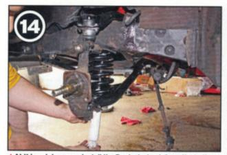
▲At this point, we can install the Doetsch shock from the bottom. It uses the factory hole in the frame and comes with hardware for the lower control arm. Once again, grease all nuts and bolts and make sure the spring is in place. Usually, if the front spring is not sitting in its pocket, the shock will not go into place. I'll admit it—that is exactly what happened to me.
