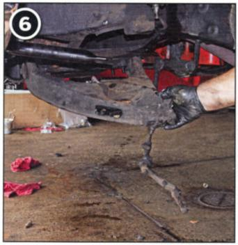
At this point, you can simply unbolt the shock, spindle, and control arms from their mounting locations. Take caution not to strip or break these bolts, as they will need to be reused. I had a bottle of Gum Cutter sitting around and hit every bolt before loosening.
