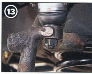
▲Once set in place, I boited the spindle in place and backed the nut off to the closest cotter pin hole. Make sure the spindle goes through the entire range of steering smoothly before you put the cotter pins in place and call it a day.
