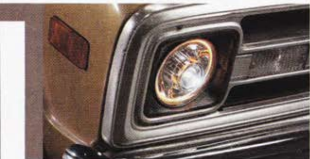
THE GRILLE IS STOCK 1970 CHEVY, BUT THE HEADLIGHTS ARE DEFINITELY NOT. HID PROJECTORS' XENON HEADLIGHT HOUSINGS ADD MODERN LOOKS WITH INCREASED SAFETY.
