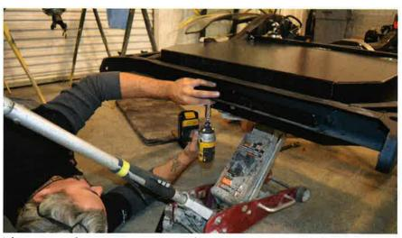
The rear tank mount uses a reinforcement bar for final installation. No worries of pulling through the frame on the rear.
