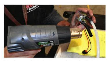
There's a couple tricks to assembling the fuel pump assembly, one of which being that heating the transfer hose will allow it to slide onto the barbed fitting on the fuel pump with relative ease. This type of connection will provide an OE-quality seal that won't leave you stranded on the side of the road.
