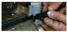
the filter/regulator mounted, we're onto fuel lines. CPP's fuel kit uses push-lock hose and AN-Style fittings throughout. Assembly is as simply as gets: insert the fitting into a vise, cut your hose to length, and push your hose on. The one-way barbs on the fitting will hold it in place for good. If they give you any trouble, a little heat applied to the hose generally makes them easier to work with
