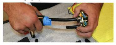
With proper depth measured, and the fuel sock installed on the pump, a good mock up and final overall measurement before cutting the transfer hose is always a good call. This measurement is also crucial for the return hose, as making it too short can cause aeration.
