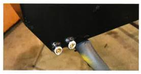
If you're using this tank in a carbureted application, or with an in-line EFI fuel pump, CPP provides you with feeds to do so. We're doing an in-tank setup for longevity and quiet operation, so we plugged these off.
