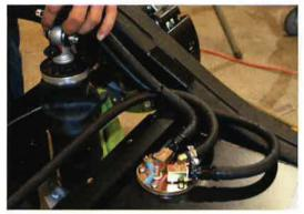
With your hoses made, the screw on just the same as any other AN fitting. Keep in mind, these are aluminum fittings; they need to be tight, but overtightening can easily strip the threads. Don't kill 'em! At this point, if you'd been working on the tank on the floor up til now, you'd want to go ahead and re-install. CPP also provides all you'll need to connect the factory filler neck to your new tank, with only slight modification required to the neck itself.
