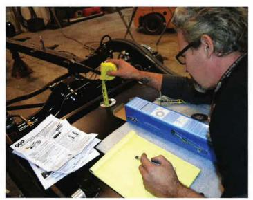
With the tank mounted, we move on to mounting the fuel sender. This is a universal piece that CPP uses in multiple applications, so some amount of application-specific modification is required. Joe starts by measuring the depth of the tank, so we know how long to adjust the unit to.
