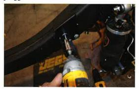
With your mounting holes drilled, front crossmember brackets are installed. These mounts are made plenty beefy, remember, that's 175lbs of fuel you'll be carrying around!
