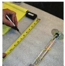
With the depth measurement taken, and the height of the level resistor determined, we can figure how long the float arm needs to be shortened to. The level sender itself is adjustable via-set screws.
