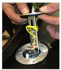
With the sending unit finalized, it gets slid into the tank. If the body was on, you'd want to install your lead and ground wires now, as once you lift the tank in place, they won't be accessible.
