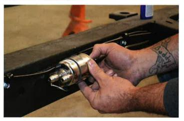
Being as the giveaway car is LS3 powered and won't require any deviation in fuel pressure away from stock, we opted to use a Vette-style filter/regulator assembly. By running the filter and regulator as one assembly, it eliminates an unsightly fuel pressure regulator in an otherwise spotless engine bay, and keeps return hose length to a minimum just the same. It's really a winwin, and all you have to do is find a good spot on the fuel rail to mount it.
