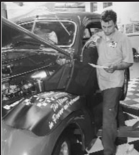
Conti then filled the system, checked for leaks, then tried the car out on the rack before lowering it.
