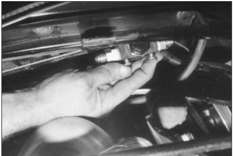
**Then he determined a suitable location for the valve. The valve can be mounted any direction with any orientation, as long as the smaller passage is the pressure side and the larger is the return/bleed-off side. It just so happened that the valve fit within arm's reach in the engine compartment.**
