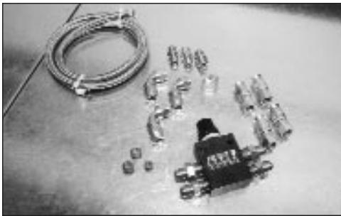
**We laid all the components out and took an inventory. There's enough -6 Teflon-lined stainless-braided hose to fit most applications. There are also 1/4-, 3/8-, 1/2-, and 5/8-inch fittings and brass seat adapters to fit most GM/Ford applications.**
