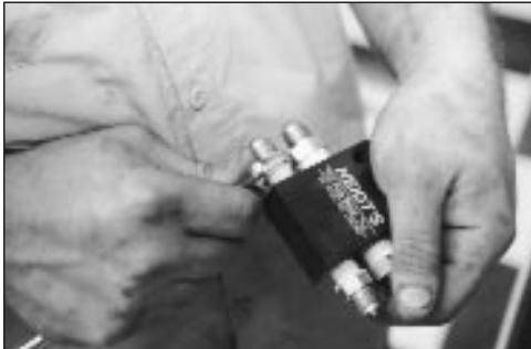
**Conti wrapped the steel fittings with sealant tape and screwed them into the block itself. Familiarize yourself with the different-sized fittings beforehand to ensure the valve gets installed with the correct orientation.**
