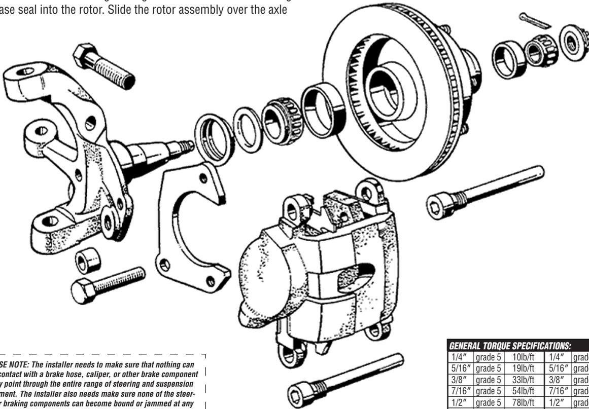
**PLEASE NOTE:** The installer needs to make sure that nothing can make contact with a brake hose, caliper, or other brake component at any point through the entire range of steering and suspension movement. The installer also needs to make sure none of the steering or braking components can become bound or jammed at any time through the range of suspension or steering movement.
