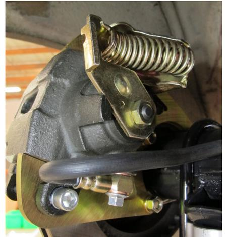
1. First verify emergency brake lever requires adjustment by checking the amount of slack (play); disconnect and remove E-brake cable and by hand, move lever in the direction of actuation, towards the front of the vehicle. If more than 1/8" of play, perform the following procedure. (Fig. 2)
