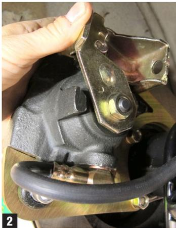
2. Remove the nut, lever, seal, and nylon washer from the parking brake adjusting screw on the caliper. (Fig. 3 & 4)
