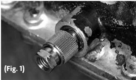
**3.** Install the splined bushing onto the transmission selector shaft, make sure the flats on the splined bushing slide over the flats on the transmission selector shaft. The kit also includes one 10mm metric nut and one standard 3/8-16 nut. Use the proper nut for your application. Tighten the splined bushing onto the transmission selector shaft (fig. 1).
