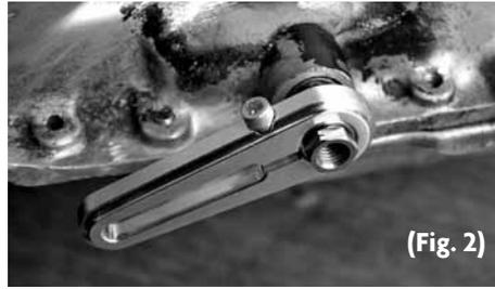
**4.** Install the aluminum arm over the splined bushing while in the 8 o'clock position (park). It may be necessary to reposition the aluminum arm per application (fig. 2).
