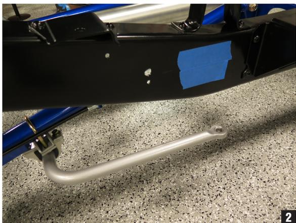
2. Attach the end links with frame brackets onto the bar, and with the bar as parallel to ground as possible, set the links at 90 degrees (perpendicular) in order to locate and mount the brackets to the framerail. (Figs 2-3)
