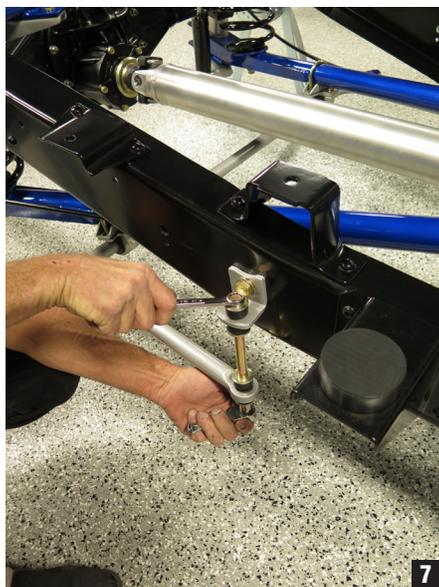
3. Mark the side of the framerrail in preparation for drilling a 7/16" hole in order to mount the end link bracket. On lowered trucks, the bracket will need to mount in the opposite direction. (Figs 4-6)
