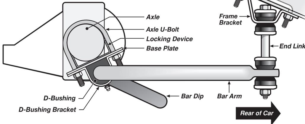
3. Before mounting the end-link frame brackets, adjust the bar position relative to the axle if needed. The axle clamp assembly holding the bar should be tilted slightly to the rear of the axle (illustrated below). The bar mid-section should run below and to the rear of the axle. It should also pass just below and to the rear of the brake junction fitting, but forward of any shocks mounted to the rear of the axle.
