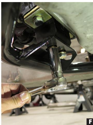
5. Install transmission with new tailshaft mount. (Figs E-F)
