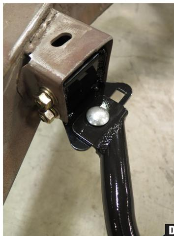
2. Unbolt and remove the factory stamped-steel transmission crossmember. (Figs A-B)
