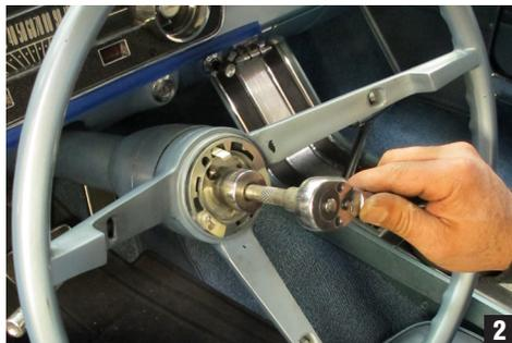
Remove the steering wheel retaining nut and set aside with the horn contact spring. These will be reused when the reassembly is done. (photo 2)
