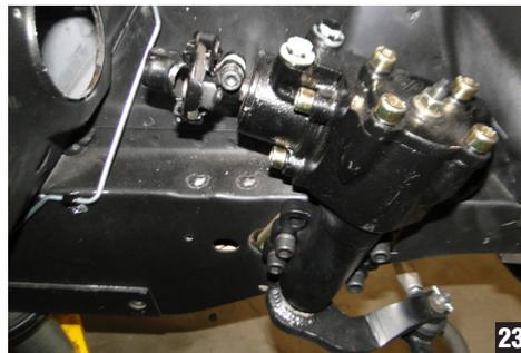
Install the rag joint onto the steering box. Remove the Allen head bolt from the rag joint and slide it onto the shaft; when the opening is visible through the hole in the rag joint put the Allen bolt back through and tighten it up. Make sure it is tight enough to remove any slop. (photo 23)
