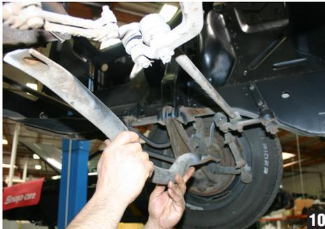
With the steering linkage and pitman arm loose it's now recommended to take the stock crossmember off temporarily to allow the steering box to be removed as one piece. This crossmember is bolted to each side of the frame so remove the hardware on each side and pull the crossmember out. This is reinstalled once the steering box is out of the car. (photo 10)
