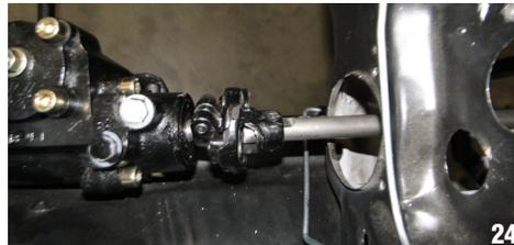
Slide the modified steering shaft back into place into the rag joint from the dash out through the firewall and leave it setting loose for the time being. (photo 24)
