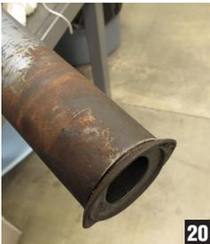
Once cut remove any sharp points or slag with a file so you can reinstall the lower column collar/seal. (photo 20)
