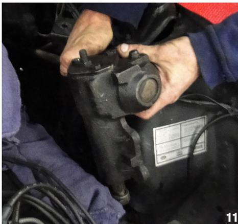
From the wheel well position remove the stock mounting bolts to the steering box. Make sure to hold the gear box when removing the last bolt so you don't drop it out as the inner steering shaft inside the car could cause damage to the dash. Once loose carefully lower the steering box out of the engine bay down from the bottom of the car. (photo 11)
