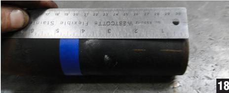
Measure 4-9/16" up from the base of the column tube and mark this point. Using blue painters tape wrapped on the column tube will make this step easy to see. (photo 18)
