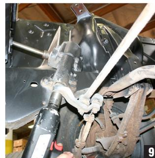
With the car securely up on jack stands, ramps or a lift now it's time to remove the pitman arm from the steering linkage and off the steering box. Using an
