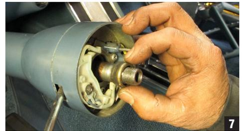
There is a small cone shaped bushing used to center the column tube from the factory. This needs to be pulled out to allow the outer column tube to be removed from the car. This part is also used again for reassembly. (photo 7)
