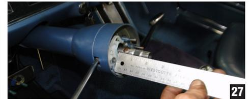
U-bracket. Snug this up just enough to keep the column from moving up or down on its own and confirm your inner shaft measurement is the same as what it was before removal in your column originally. (photo 27)
