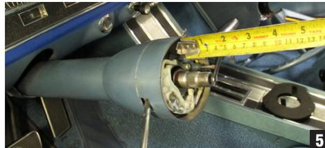
Before you remove the steering column out of the car take a measurement of how much inner steering shaft protrusion come out at the top of the column; this measurement (approximately 3") is to be used when you cut the steering shaft later in the instructions to ensure the steering wheel seats properly without bottoming out on the steering column. (photo 5)
