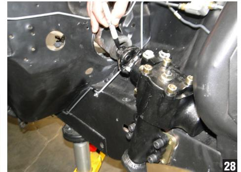
Once you confirm your upper measurement now is time to mark and drill the roll pin hole. If you can accomplish this while in the car you can simply drill the hole. If you have limited space simply remove the inner shaft again and drill it out with a drill press. (photo 28)
