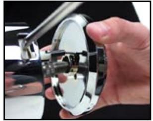
top of the column with those in the adaptor and slide it onto the column. A nut has been provided with your steering column. The nut will secure the wheel to the top of the column. The nut on the wheel should be torqued to 40 ft lbs.
