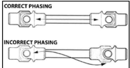
5. Sometimes if the u-joints are at a severe angle, even if they are phased correctly, a hard spot in the steering may occur for no apparent reason. If this happens, index the u-joints two or three splines in one direction. The hard spot should disappear or be minimized.
