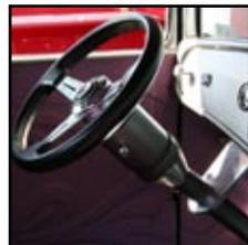
**It is highly recommended that you test fit your steering column before painting the column. Test fitting now will save you a headache later on. We are not responsible for paint.**
