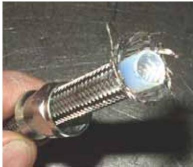
**Step Five:** Grab the hose and push it firmly against a solid surface to push the teflon liner all the way into the ferrule until it seats against a flat inner stop.
