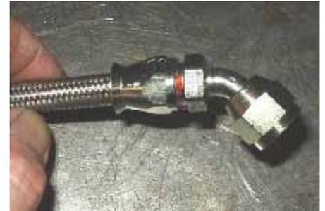
**Step Eleven:** Using your favorite cleaner spray or hot soapy water, flush the assembled hose of any possible debris, then blow out the hose with compressed air.
