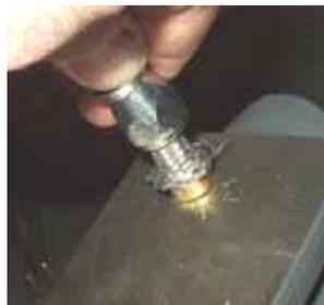
**Step Six:** Grab a suitable tapered punch and expand the teflon liner into the I.D. of the ferrule firmly.
