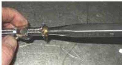
**Step Seven:** Put a few drops of your favorite lube on the hose end male nipple, the threaded area of the hose end, and a drop also in the female hose end to aid assembly and prevent thread galling while tightening. (Any lube will essentially do, though we prefer to use the moly cam / lifter assembly lube here in house).
