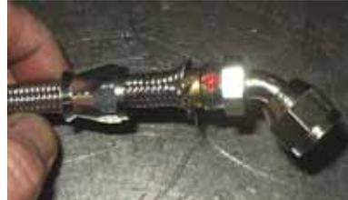
**Step Nine:** Slide the female hose nut firmly up and over the necked out stainless hose over braid until you can get the hose end threaded into the nut - be careful not to cross thread these two items.
