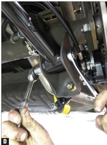
4. Reusing the original hardware, install the new CPP Totally Tubular arm: the threaded bungs (on the rear pivot end of the arm) will point toward the drive shaft. (Fig. B, C, D)
