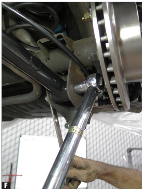
7. Torque 12mm trailing arm pivot bolts to 70lb/ft. (Fig. F)
