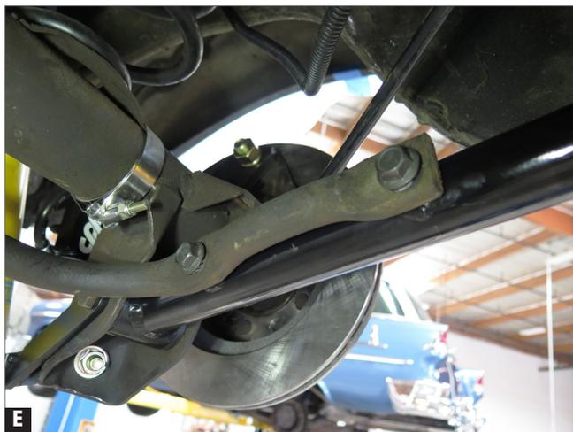
6. To reinstall stock sway bar, attach using supplied M10-1.5x35mm flanged head bolts and serrated lock washers. (Fig. E)
