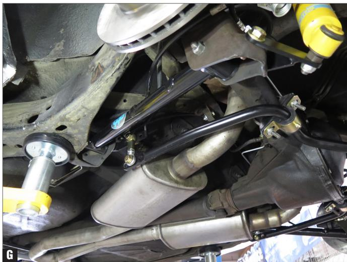
8. CPP's Pro Touring Sway Bar (#7887PTSBK) will not mount off the new trailing arms, as it uses a separate mounting bracket for the adjustable end links. (Fig. G)
