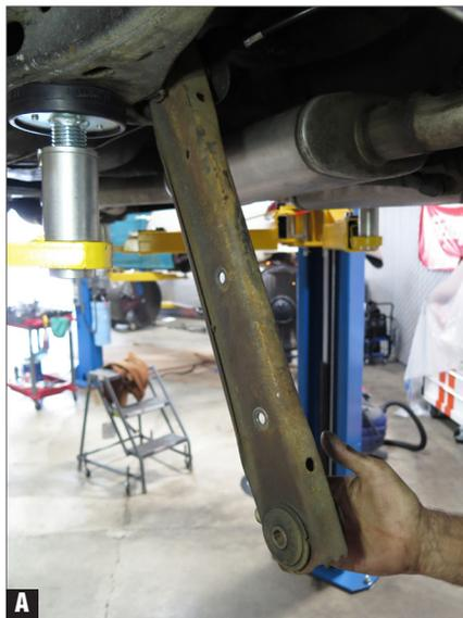
3. Unbolt and remove one stock lower arm; swap one at a time to prevent excess movement of rear end. (Fig. A)
