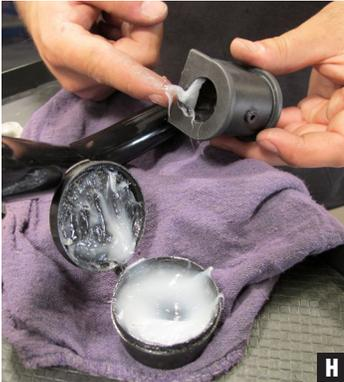
8. Coat the sway bar pivot/D-bushings with grease and install onto sway bar. (Fig H)
