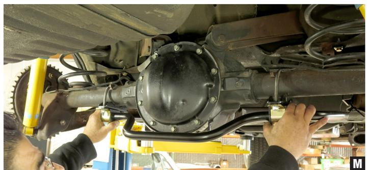
12. Rotate axle clamps until link ends are perpendicular to the ground, without sway bar contacting rear end. (Fig M)
