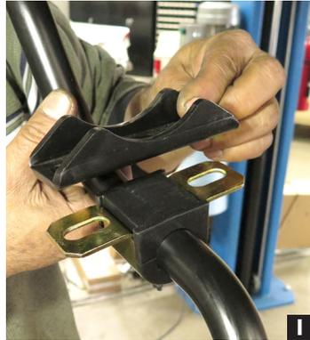
9. Set the sway bar mounting brackets onto the bushings centering the nipple into the zerk fitting hole; don't forget to install zerk fittings into the clamps. (Fig I)
