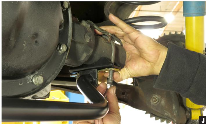
10. Install the axle clamp U-bolts onto rear end housing beneath the brake lines; take care not to damage lines. Connect sway bar with D-bushing bracket and lower axle clamp. Dip in bar will be down and towards the rear. (Fig J)
