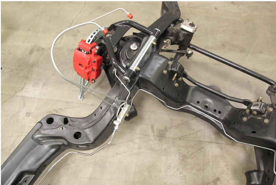
**PLEASE NOTE:** The installer needs to make sure that nothing can make contact with a brake hose, caliper, or other brake component at any point through the entire range of steering and suspension movement. The installer also needs make sure none of the steering or braking components can become bound or jammed at any time through the range of suspension or steering movement.
