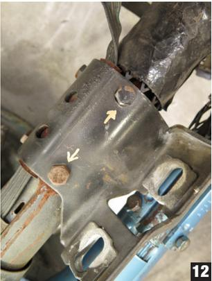
12. If the upper column bracket will not adjust enough, oblong the holes attaching it to the column until it does.
