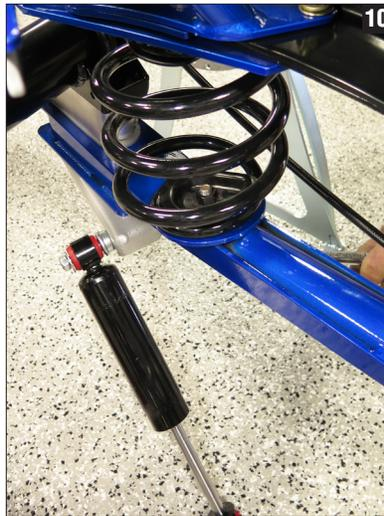
10. With the shock attached to the lower mount, reinstall the coil spring; the upper pocket will use the supplied hardware to attach and secure the shock crossmember. (Fig 10)
