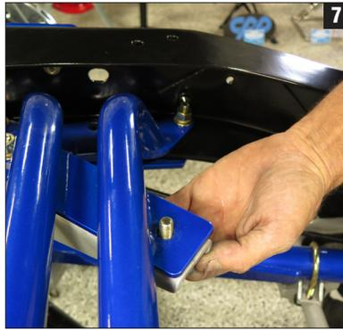
7. Note: bolts (at least the rear one) must be inserted from the bottom so as to not interfere with the shock absorber itself. (Fig 7)
