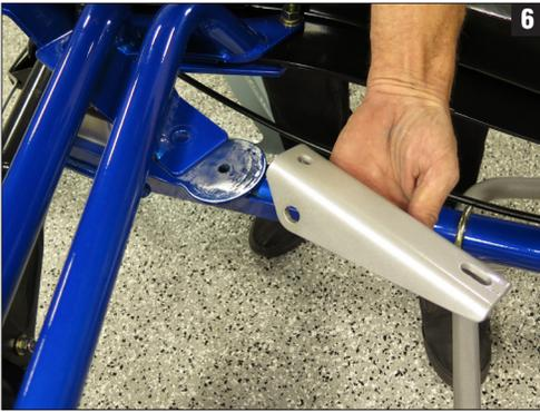
6. Install the upper Shock Relocater bracket with the slotted hole forward; the shock will mount at the rear side of the bracket. (Fig 6)
