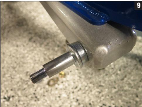
9. CPP offers new lower shock studs (CPP-SMS) as well as three shock options: (CPP-4163G) stock; (CPP-4095G) 2-4" lowered; and (CPP-4052G) 5" lowered. (Fig 9)
