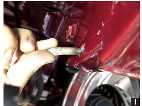
9. Insert the U-bolt through the holes so that the threaded ends stick through the frame on the inside sections first. (Fig I)
