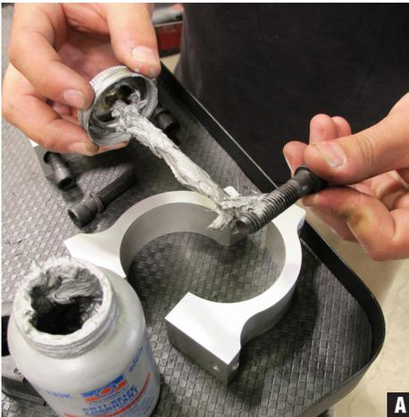
2. For billet axle clamps, coat socket head Allens with antiseize. (Fig A)
