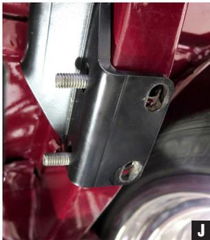
10. Attach bracket with the end links still connected; install nyloc nuts finger tight. (Fig J)
