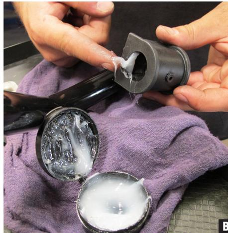
3. Coat the sway bar pivot/D-bushings with grease and install onto sway bar. (Fig B-C)
