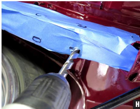
8. Remove the bracket and drill 3/8" holes on the bottom and inside of the frame. (Fig H)
