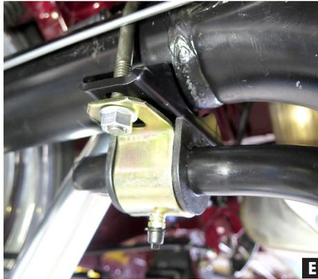
5. Install standard axle clamp U-bolts onto rear end housing; connect sway bar with D-bushing bracket and lower axle clamp. Dip in bar will be down and towards the rear. (Fig E)
