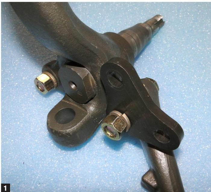
2. Un-bolt the factory steering arm from the spindle. Using the new hardware, bolt the small three hole bracket to the back of the steering arm. Do not tighten at this time. (Photo 1)
