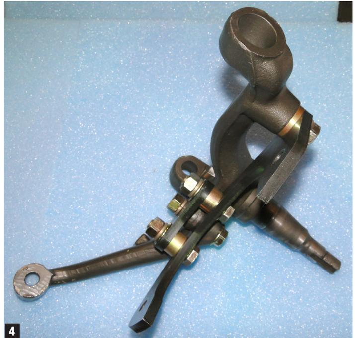
**PLEASE NOTE:** The installer needs to make sure that nothing can make contact with a brake hose, caliper, or other brake component at any point through the entire range of steering and suspension movement. The installer also needs to make sure none of the steering or braking components can become bound or jammed at any time through the range of suspension or steering movement.
