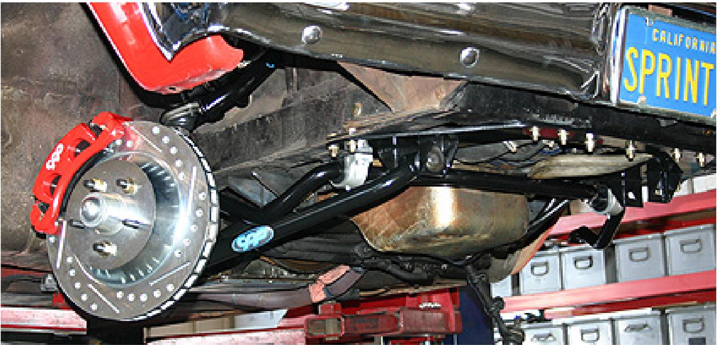
**PLEASE NOTE:** The installer needs to make sure that nothing can make contact with a brake hose, caliper, or other brake component at any point through the entire range of steering and suspension movement. The installer also needs make sure none of the steering or braking components can become bound or jammed at any time through the range of suspension or steering movement.
