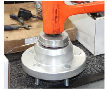
6. Pack the wheel bearings with grease. Install the inner bearings and the grease seal. Install the hub assembly. Install the outer wheel bearing, washer and spindle nut. Adjust the wheel bearings as follows:
