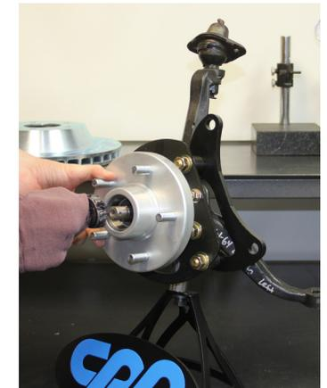
**PLEASE NOTE:** The installer needs to make sure that nothing can make contact with a brake hose, caliper, or other brake component at any point through the entire range of steering and suspension movement. The installer also needs to make sure none of the steering or braking components can become bound or jammed at any time through the range of suspension or steering movement.
