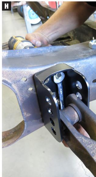
5. Attach the CPP Anti-Squat brackets using the supplied Grade 8 hardware. (Figs G-H)
