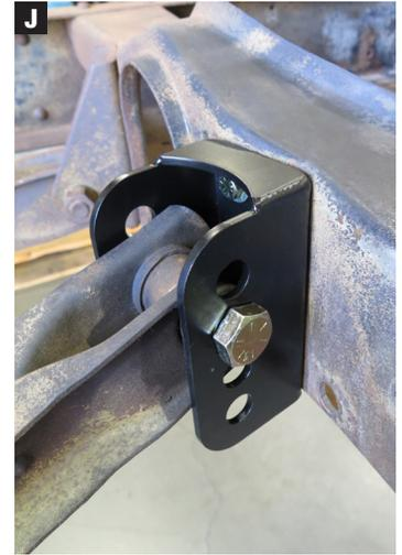
6. Reconnect the trailing arms; use the mounting hole that best corresponds with the amount the rear end has been lowered (the lower the suspension, the higher the mounting hole) to properly set your pinion angle. (Figs I-J)
