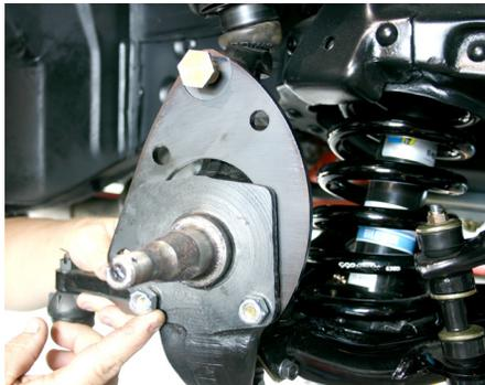
3. Install the caliper bracket behind the "A" shaped bracket with the spacer
