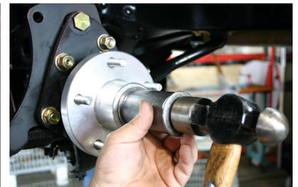
6. Install the dust cap. Slide the rotor onto the hub and secure with a couple lug nuts. Note: There is a left and right rotor. The holes and slots will be turning in a clockwise rotation.
