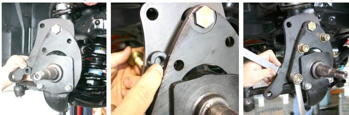
ers placed between the two brackets as shown. Tighten down these three bolts.
