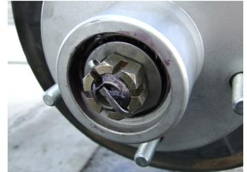
drag. Install the cotter pin and dust cap. *(Note: We removed the brake hardware to better illustrate the installation.)*
