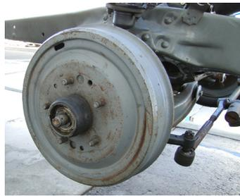
3. Clean and inspect the spindle pin. Be sure to remove the old style bearings and race. Check for any rough or worn spots on the spindle pin. Also note, sometimes the old ball bearing race will freeze up on the spindle pin. Use care in removing it as not to damage the spindle pin.
