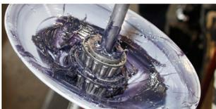
5. Pack good quality bearing grease into the new CPP roller bearings. Place the inner bearing into the back side of the CPP aluminum hub.
