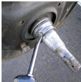
4. Next, remove the factory iron hub from the brake drum. Original drums are riveted together and you will need to grind the rivets to separate the hub from the brake drum.
