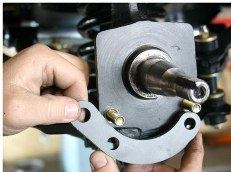
1. Start by removing either the factory drum brake assembly or your current disc brake conversion from the stock spindle. This would be a good time to inspect the spindle, ball joints and tie rods for any wear issues.
