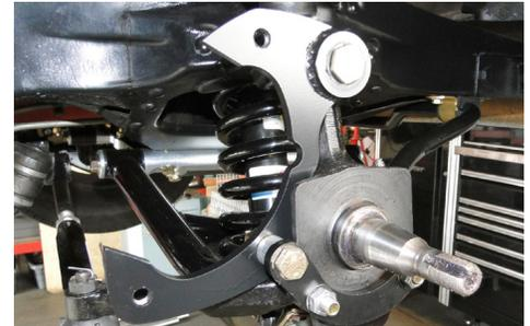
Tighten down the top anchor bolt and bracket bolt now.
