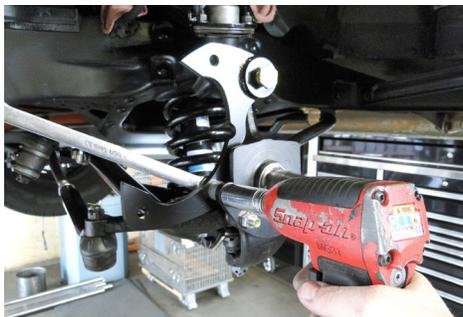
3. Install the small spacer between the small bracket and the large caliper bracket as shown in the picture. Leave the bolt loose at this time.
