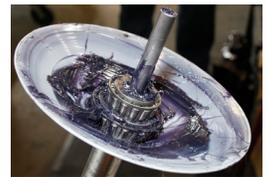
Install the rotors onto the spindle, then the outer bearings, spindle washers, and the new spindle nuts supplied in the kit. Adjust the wheel bearings as follows:
