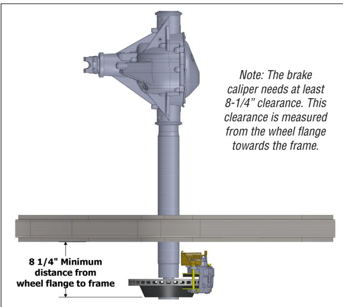
**PLEASE NOTE:** The installer needs to make sure that nothing can make contact with a brake hose, caliper, or other brake component at any point through the entire range of steering and suspension movement. The installer also needs to make sure none of the steering or braking components can become bound or jammed at any time through the range of suspension or steering movement.
