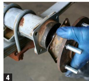
7. Slide the backing plate shim on to the axle and re-install the axles into the rear end housing. (Used on 1955-64 axles only) (Fig. 3 & 4)
