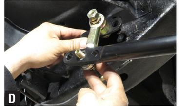
5. With the vehicle at ride height (or suspension compressed/loaded to emulate ride height), rotate the sway bar parallel to the frame and/or ground to determine where the link brackets will attach to the framerrails. On wagons, you will need to rotate the axle brackets further forward (approximately 180° from the brake line tab on passenger side) to avoid the bar hitting the fuel tank upon severe suspension compression. (Fig. E)
