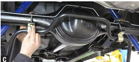
4. Assemble the Heim joint end links and loosely attach to the sway bar and frame brackets (start off with center holes). See illustration for adjustment notes. (Fig. D)
