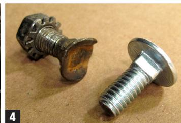
3. If the factory shock tower hardware is questionable, replace with 3/4-inch 5/16-18 carriage bolts; the heads may require slight grinding to properly fit between the sheetmetal and top of the coil spring. (Figs 3-4)
