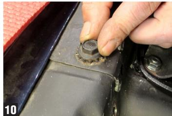
10. Securely tighten all hardware on both braces, as well as upper shock mounts.
