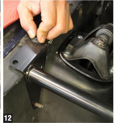
5. The top portion of the brace will bolt directly on top of the firewall/cowl seam (as opposed to beneath, as with the two-piece brace) in the existing four holes. Use a punch to help align holes if necessary. (Figs 7-8)
