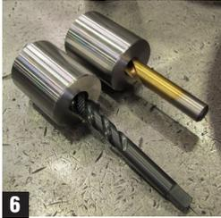
6. The bushings are machined to fit the ID of the balancer mounting hole (1.225"). The inner lip of the balancer may require slight cleaning up with a file or sand paper if it's been hammered on in the past. (Figs. 7-8)
