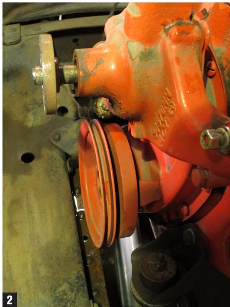
2. Removal of the early-style dampers/pulleys is no different than removing a later-style balancer (using a puller); it's the reinstallation
