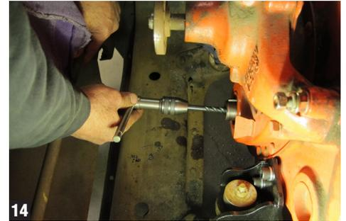
12. Always keep the tap well-oiled with cutting fluid and wipe off the metal debris regularly to ensure your crank threads are sharp and clean. Install the new balancer bolt prior to putting the balancer on to verify threads are accurate. (Fig. 15)
