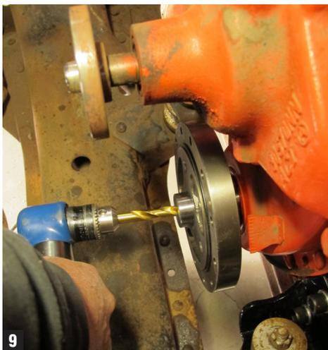
8. Start tapping the threads (using the tap bushing) once the hole has been drilled to depth; keep tap well lubricated with cutting fluid and periodically clean off debris. Cut approximately a half-inch deep, just enough to stabilize tap without bushing. (Fig. 10)
