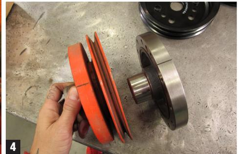
4. The existing pilot hole will initially determine how the job proceeds—if it's not deep enough, getting your drill's pilot hole dead-center may be difficult (without having to machine an addition guide to drill a pilot). Verify first before moving forward. (Fig 5)
