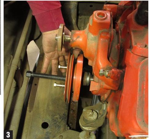
3. CPP's #18-35 harmonic balancer (6-1/8" diameter, 3/4" thick) replaces the early integrated balancer; it's slightly more offset, which benefits pulley spacing, however the timing mark matches up identically. (Fig 4)
