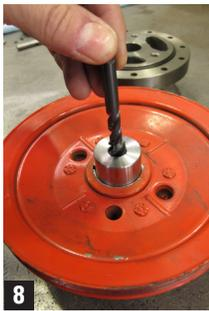
7. The preferred manner to drill and tap the crank is with the balancer still installed, as it provides more stability. Use a new, cobalt (HSCo) bit. Measure the required hole depth based on the length of your replacement balancer bolt and mark bit accordingly. (Fig. 9)
