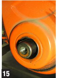
13. Use an oversized 7/16-20 bolt to initially install the balancer—make sure to avoid bottoming the bolt out (and possibly damaging the new threads) in the process. (Fig. 16)
