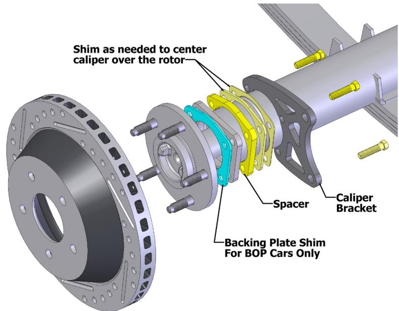
10. Install the spacer and caliper bracket
