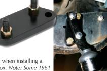
mend using the later idler arm when installing a 500 Series™ power steering box. *Note: Some 1961 models may require this bracket.*
